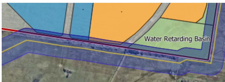
Figure 17 Southern boundary of the O'Connor land showing the pipeline alignment with a 50 metre 'buffer' 267
