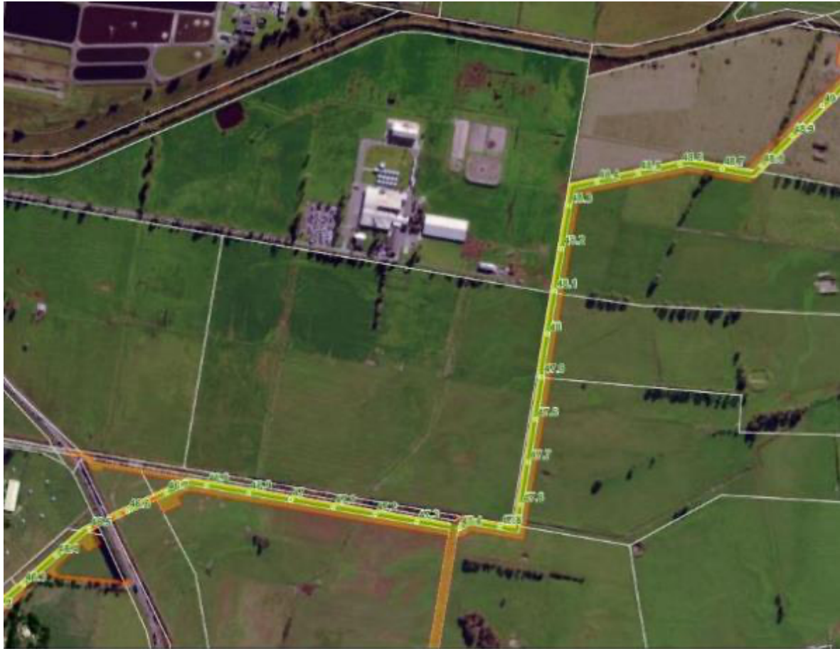
Figure 16 Proposed pipeline alignment 266
