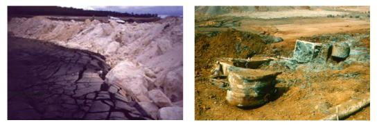
Most tailings covers follow the gentle slope (about 1%) of the tailings beach and hence are conventionally rainfall-shedding, generally towards a spillway constructed through natural high ground. If the tailings are potentially contaminating, the construction platform on soft tailings should be coarse grained and have no
