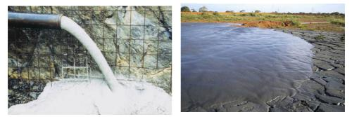
Figure 1: Paste tailings: (left) cemented underground backfill; (right) surface disposal
