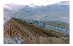
Figure 6: Dry-stacked, filtered tailings transported by conveyor and compacted by dozer
