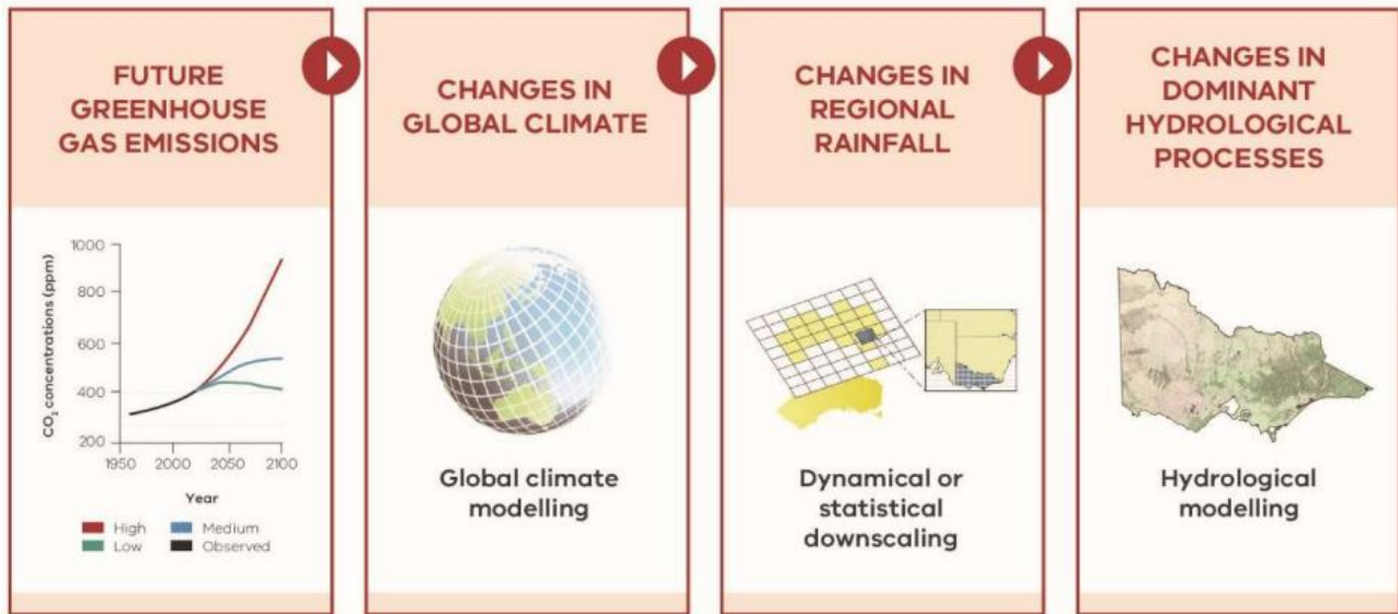
Figure 1 Overview of modelling process to derive climate change projections from global climate models (DELWP 2020)
