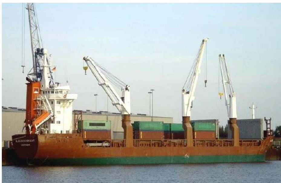
Figure 7.2 Multi-Purpose Vessel with containers
