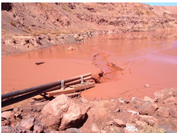
Prior to startup Tails depositing as smooth paste No beaching - No water release
