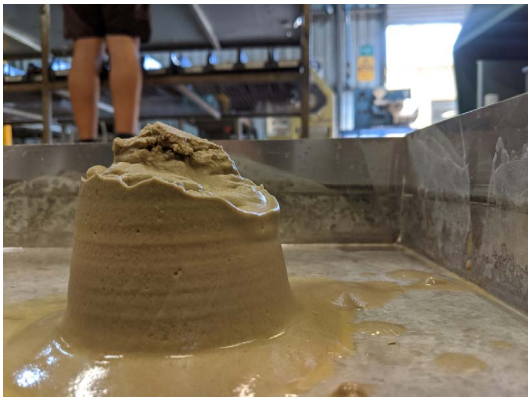
Figure 2 Fingerboards 73% coarse sand tailings after dewatering
