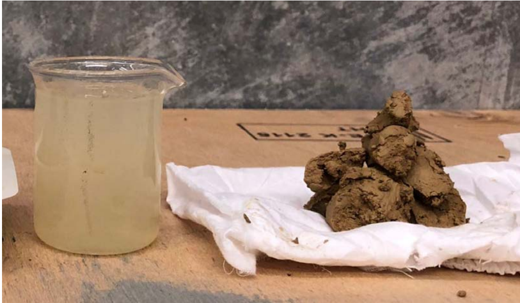
Figure 5 Centrifuged Fingerboards fines cake with centrate
