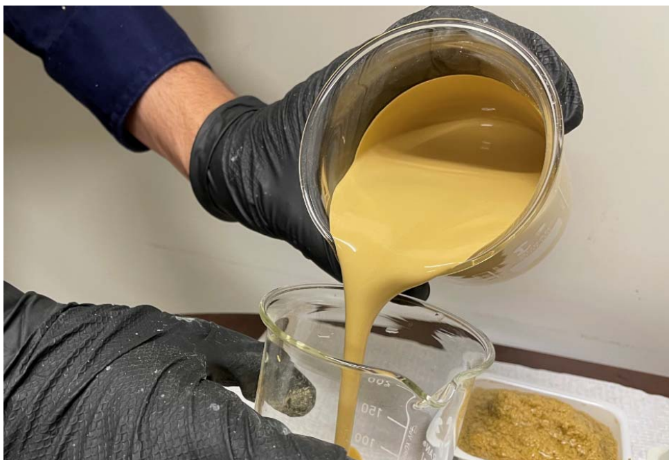
Figure 2: Sample diluted to 26.0% suspended solids
