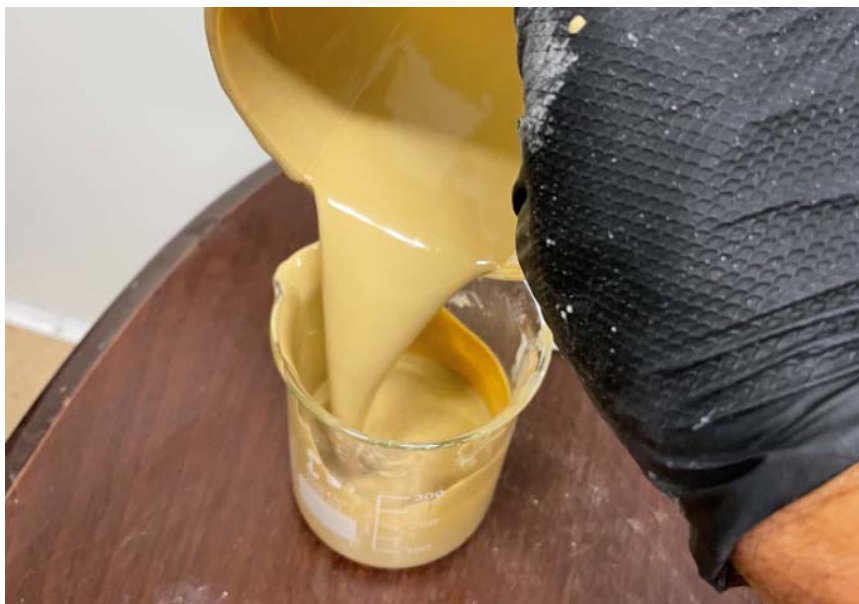
Figure 2: Sample diluted to 26.0% suspended solids
