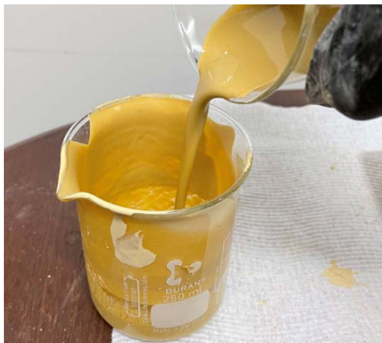
Figure 2: Sample diluted to 23.0% suspended solids
