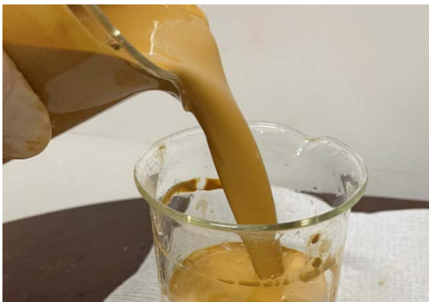
Figure 2: Sample diluted to 26.0% suspended solids
