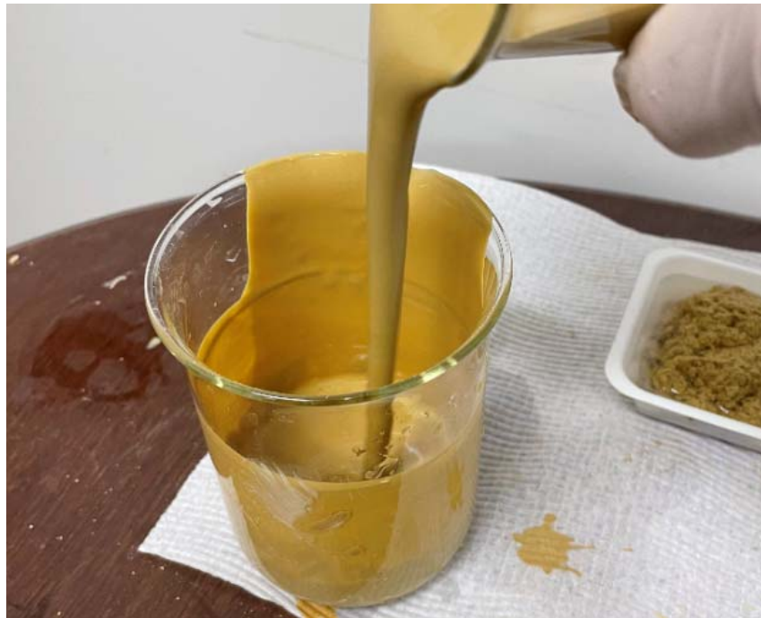
Figure 1: Sample as received at 35% suspended solids
