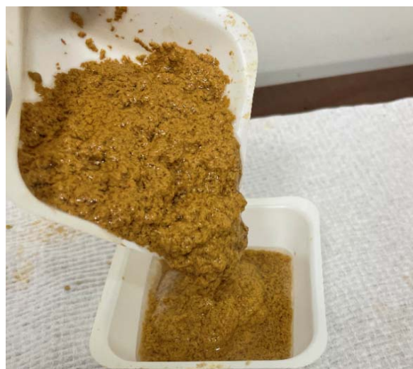
Figure 3: Flocculated solids at 26% wt suspended solids
