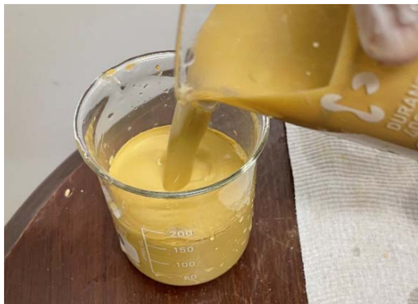
Figure 2: Sample diluted to 26.0% suspended solids
