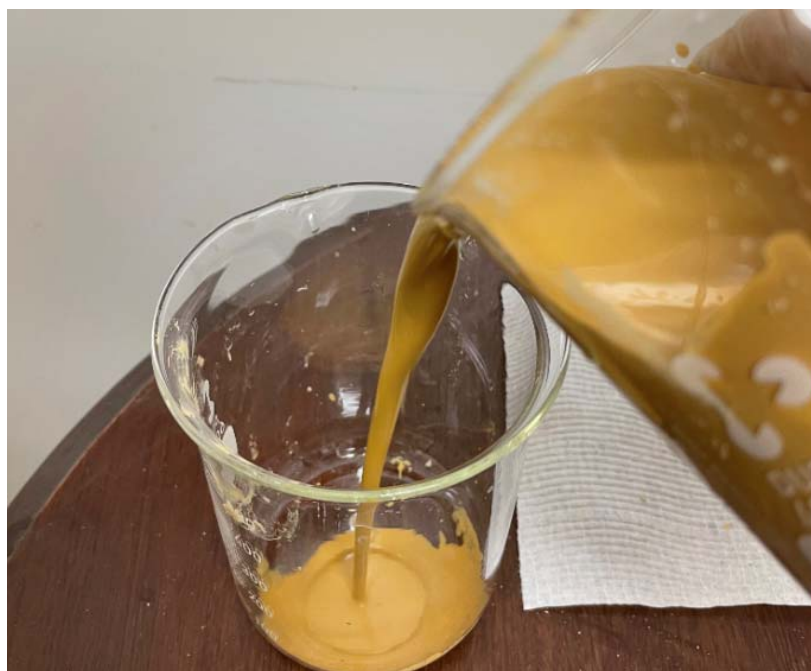
Figure 2: Sample diluted to 27.0% suspended solids
