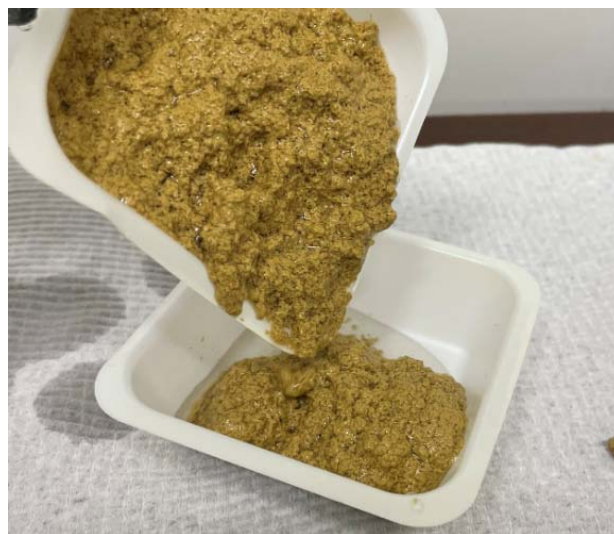
Figure 3: Flocculated solids at 26% wt suspended solids
