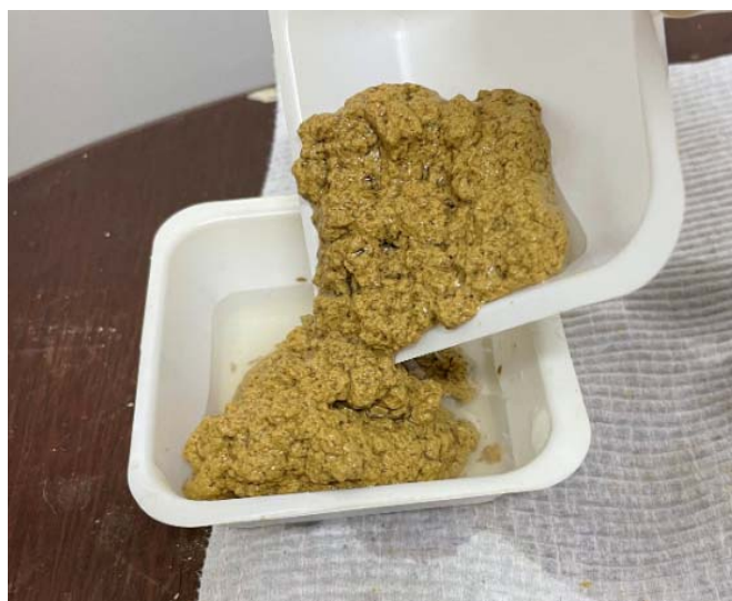
Figure 3: Flocculated solids at 27% wt suspended solids
