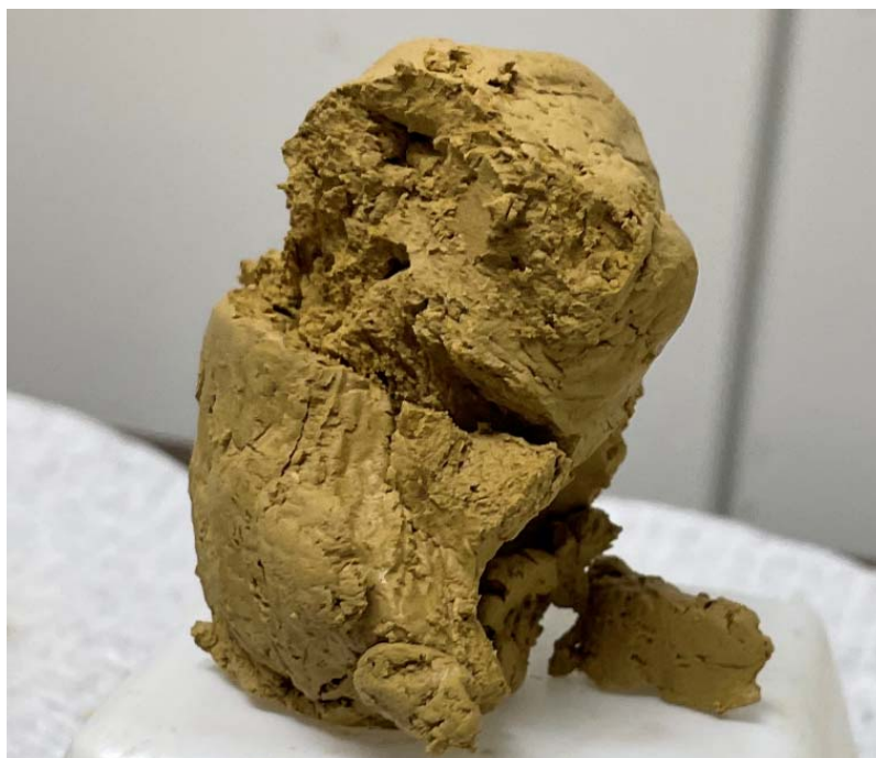
Figure 6: Cake at approximately 65% wt suspended solids
