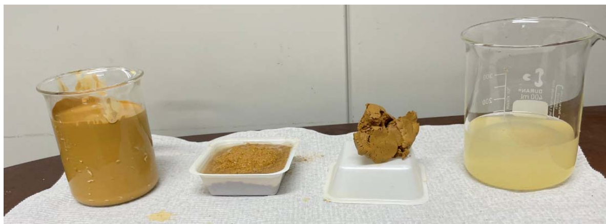
Feed (at 26% solids), flocculated feed, cake and centrate
