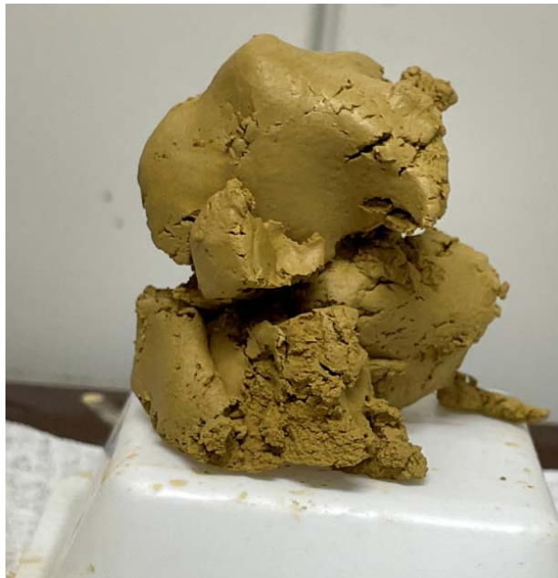
Figure 6: Cake at approximately 67% wt suspended solids
