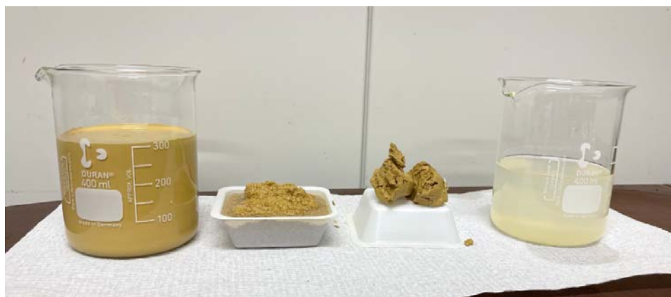
Feed (at 26% solids), flocculated feed, cake and centrate
