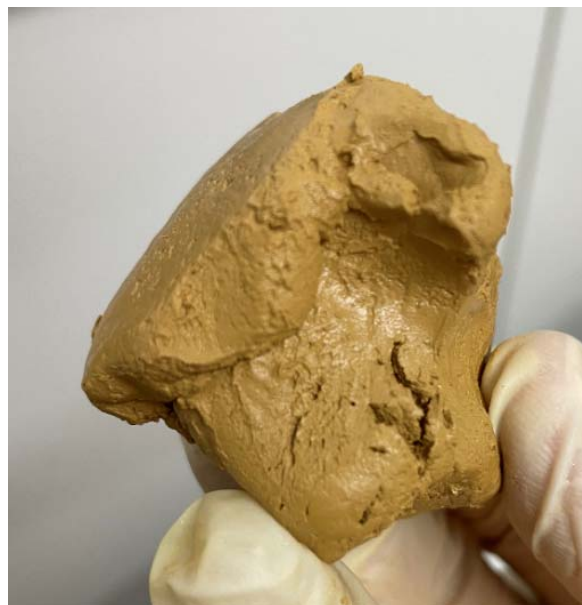
Figure 6: Cake at approximately 60% wt suspended solids
