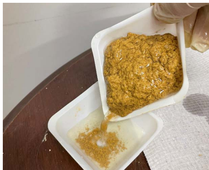
Figure 3: Flocculated solids at 27% wt suspended solids
