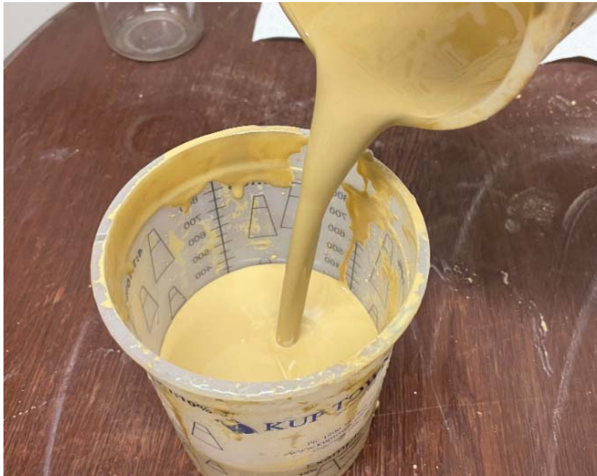
Figure 1: Sample as received at 35% suspended solids
