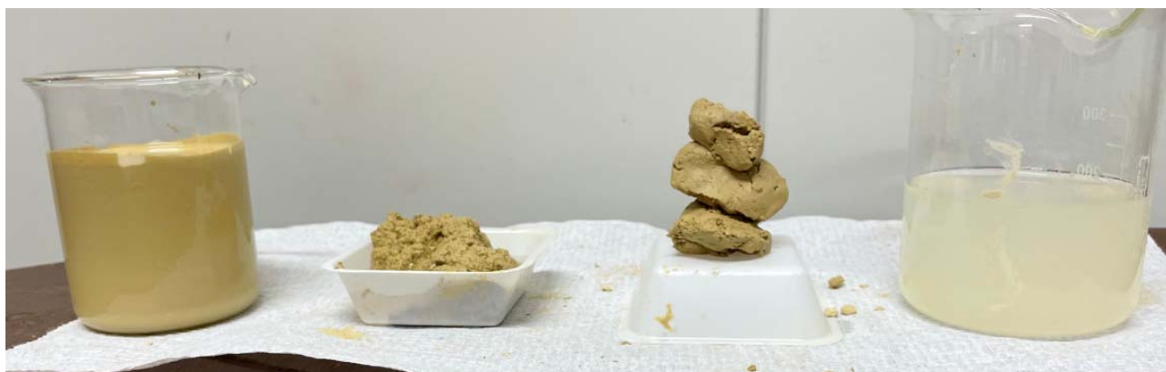
Feed (at 26% solids), flocculated feed, cake and centrate
