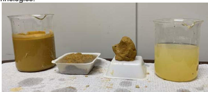
Feed (at 27% solids), flocculated feed, cake and centrate
