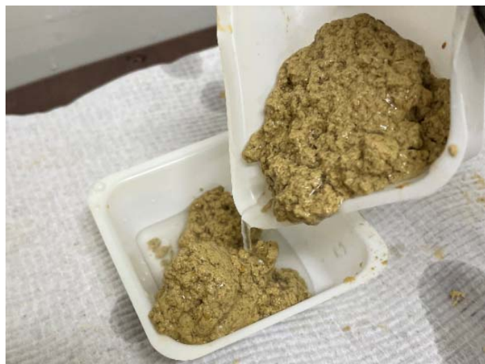
Figure 3: Flocculated solids at 26% wt suspended solids
