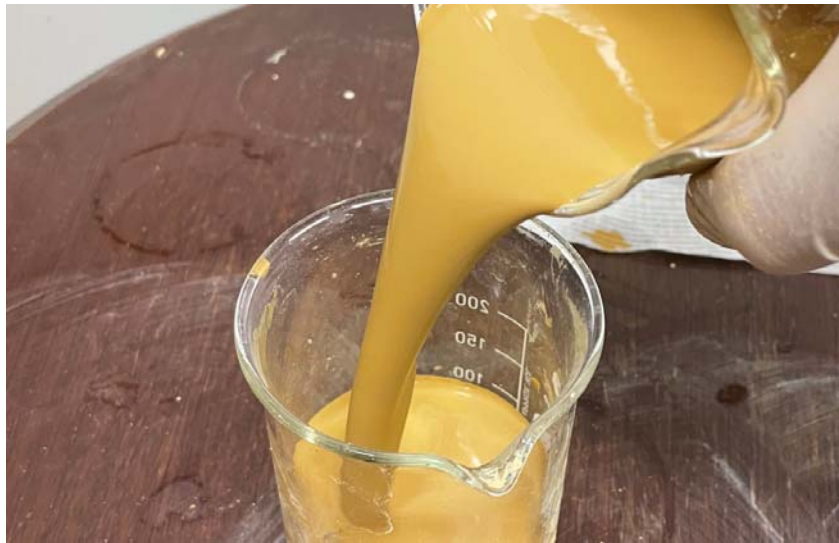
Figure 1: Sample as received at 35% suspended solids
