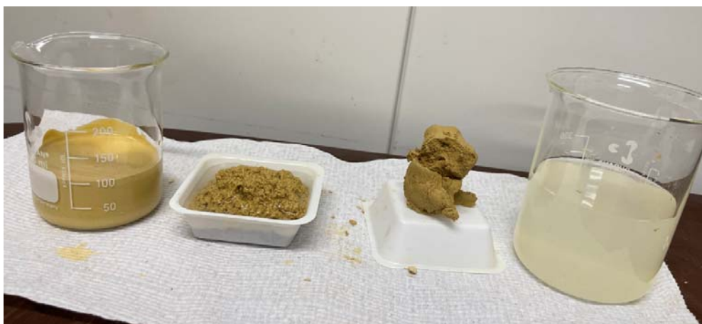
Feed (at 23% solids), flocculated feed, cake and centrate
