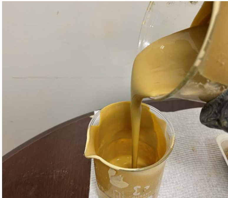
Figure 1: Sample as received at 35% suspended solids
