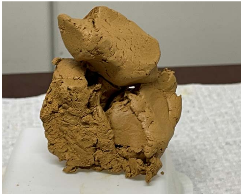
Figure 6: Cake at approximately 67% wt suspended solids
