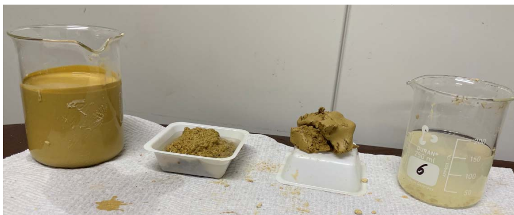
Feed (at 27% solids), flocculated feed, cake and centrate
