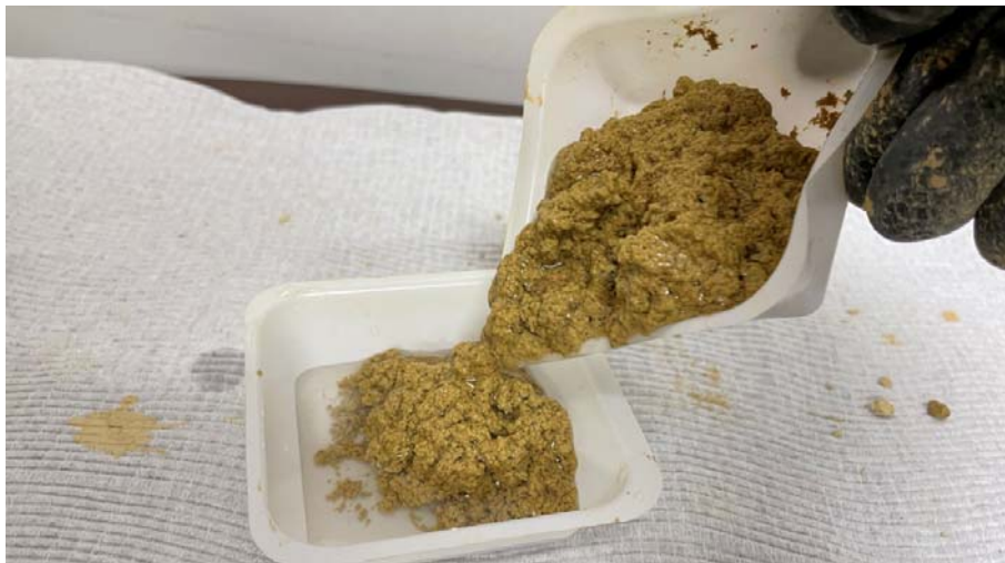
Figure 3: Flocculated solids at 23% wt suspended solids
