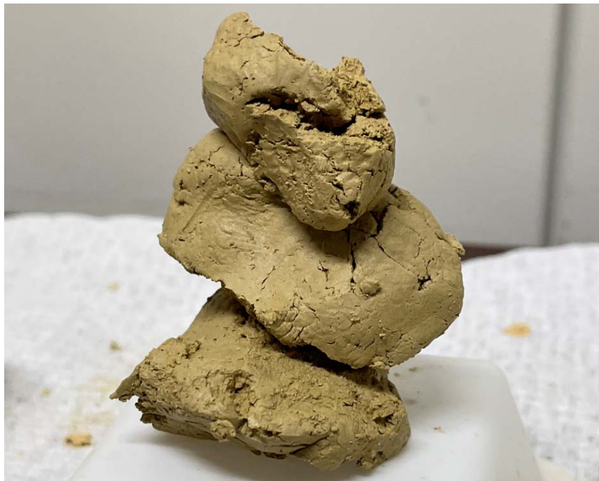
Figure 6: Cake at approximately 66% wt suspended solids
