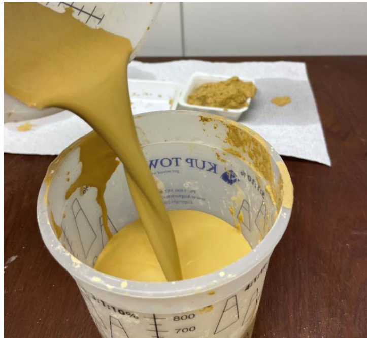
Figure 1: Sample as received at 35% suspended solids
