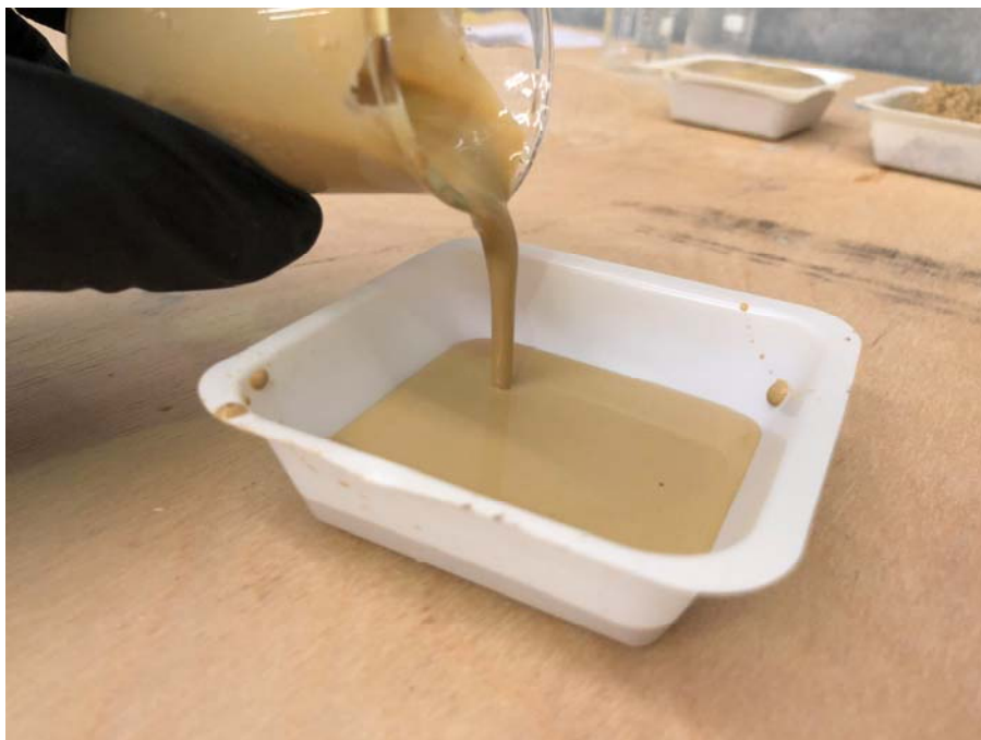
Figure 2: Sample diluted to 25.0% suspended solids
