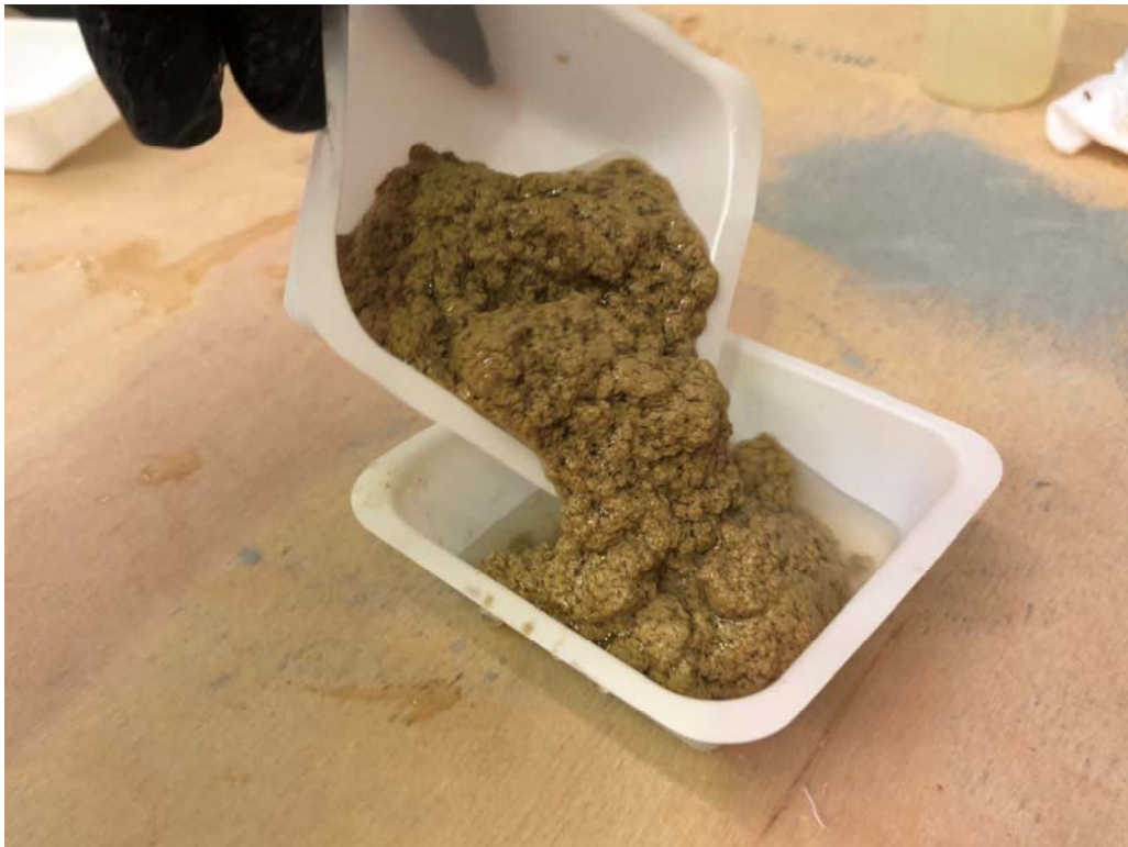
Figure 3: Flocculated solids at 25% wt suspended solids
