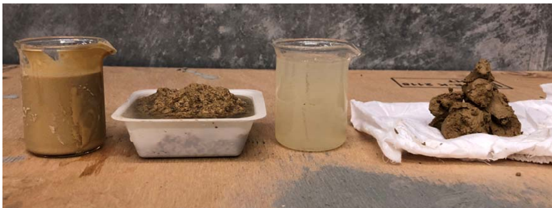
Feed (at 25% solids), flocculated feed, centrate and cake
