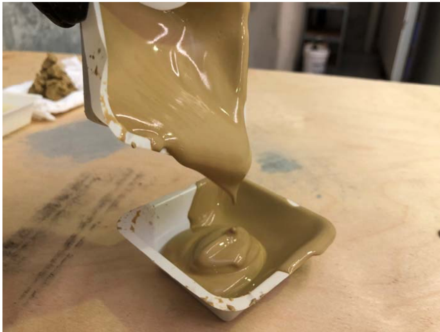
Figure 1: Sample as received at 48.2% suspended solids
