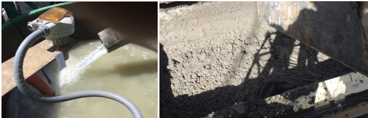
Figure 9 Liquid and solid discharge of centrifuge
