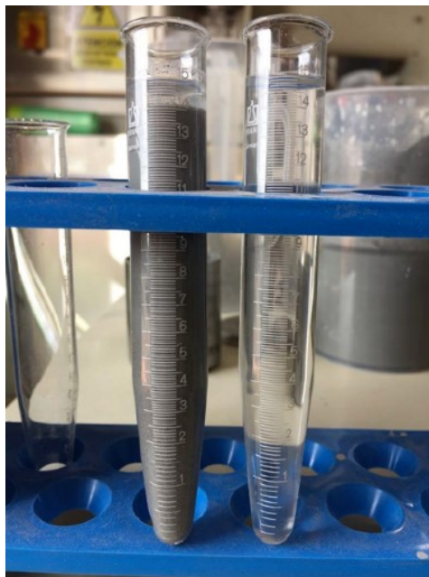
Figure 19 Feed and centrate discharge at Cuajone mine (lab test centrifuge 9,810 \text{ m/s}^2 ( 1,000 \times g ) for one minute)
