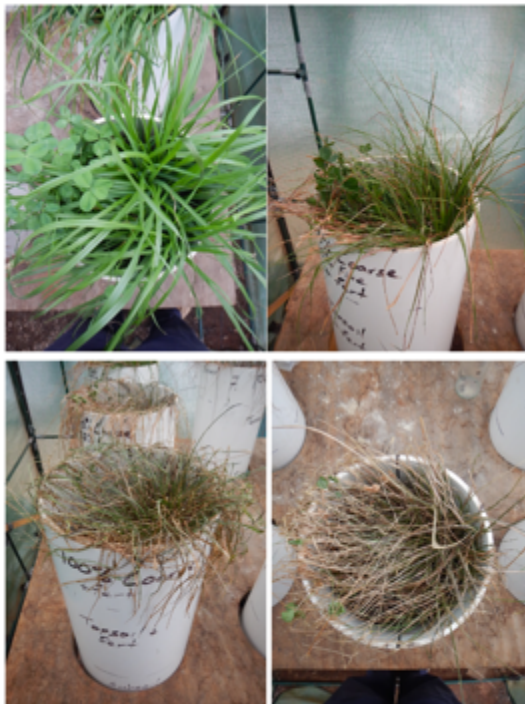
Figure 6: Condition of vegetation immediately prior to final harvest: clockwise from top left – 75%, 50%, 25% and 0% fine tailings in subsoil, all treatments fertilised.
