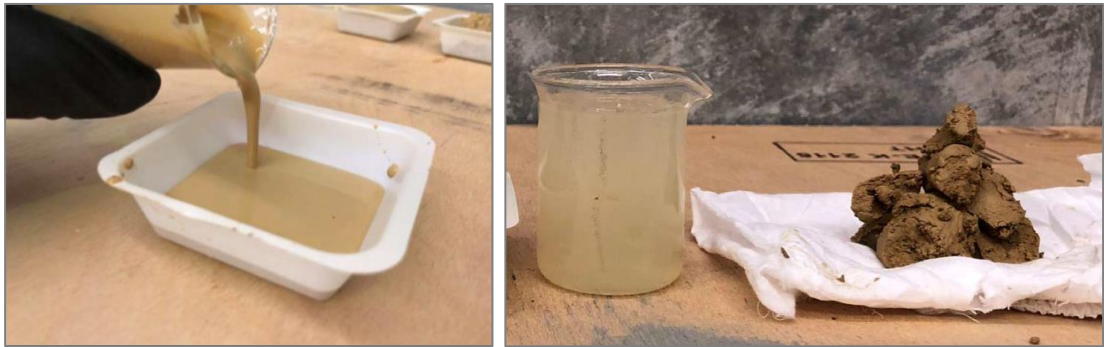
Figure 9 Left - fine tailings after thickening; 27 right – overflow water (centrate) and ‘cake’ 28
