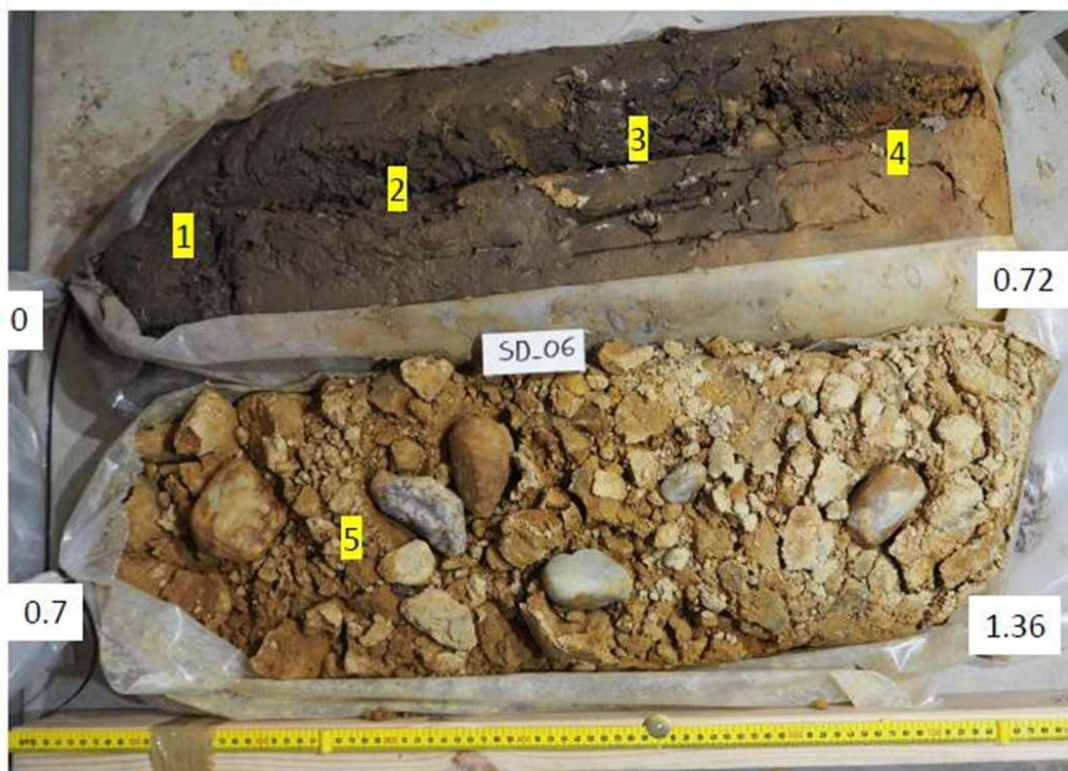
Figure 2-12: Stockdale/Munro sandy soil over clayey gravel at SD06 (529855.5mE; 5817527.8mN)
