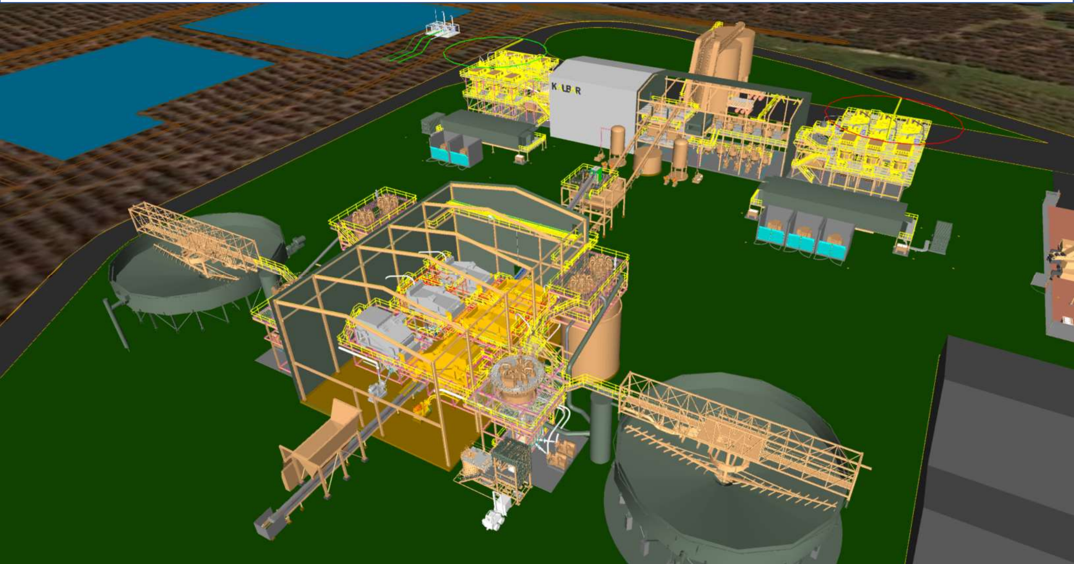
Close up view of the WCP with cladding removed for interior visibility. Screening and de-sliming building in the foreground and gravity and magnetic separation building in the background.
