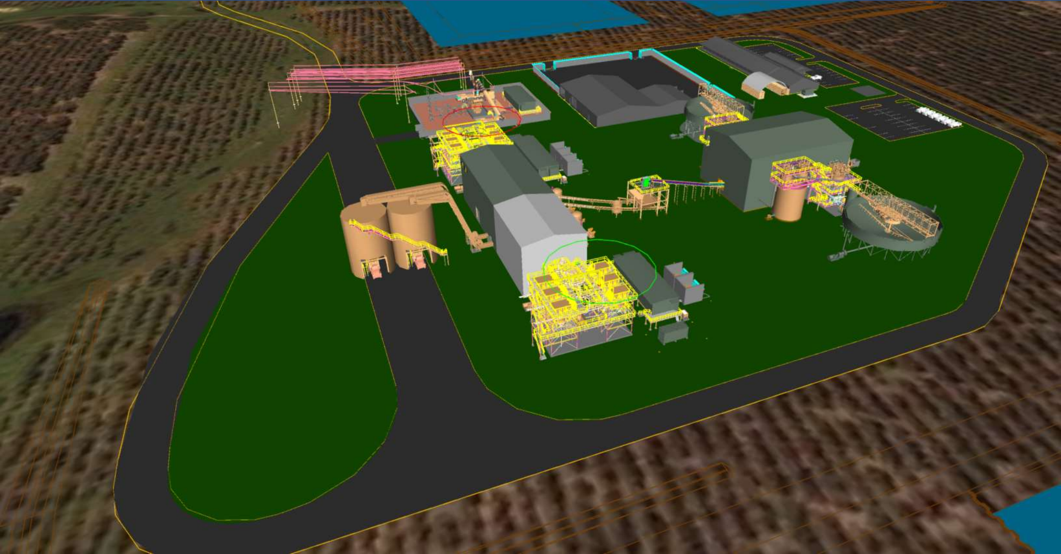
Close up view of the WCP viewed from the west. HMC storage silos for truck loading shown to the left of the magnetic separation building.
