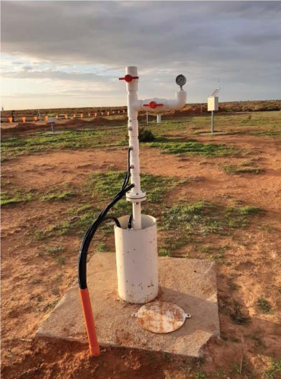
Plate 4.1 Specialised groundwater collection system – bore setup
