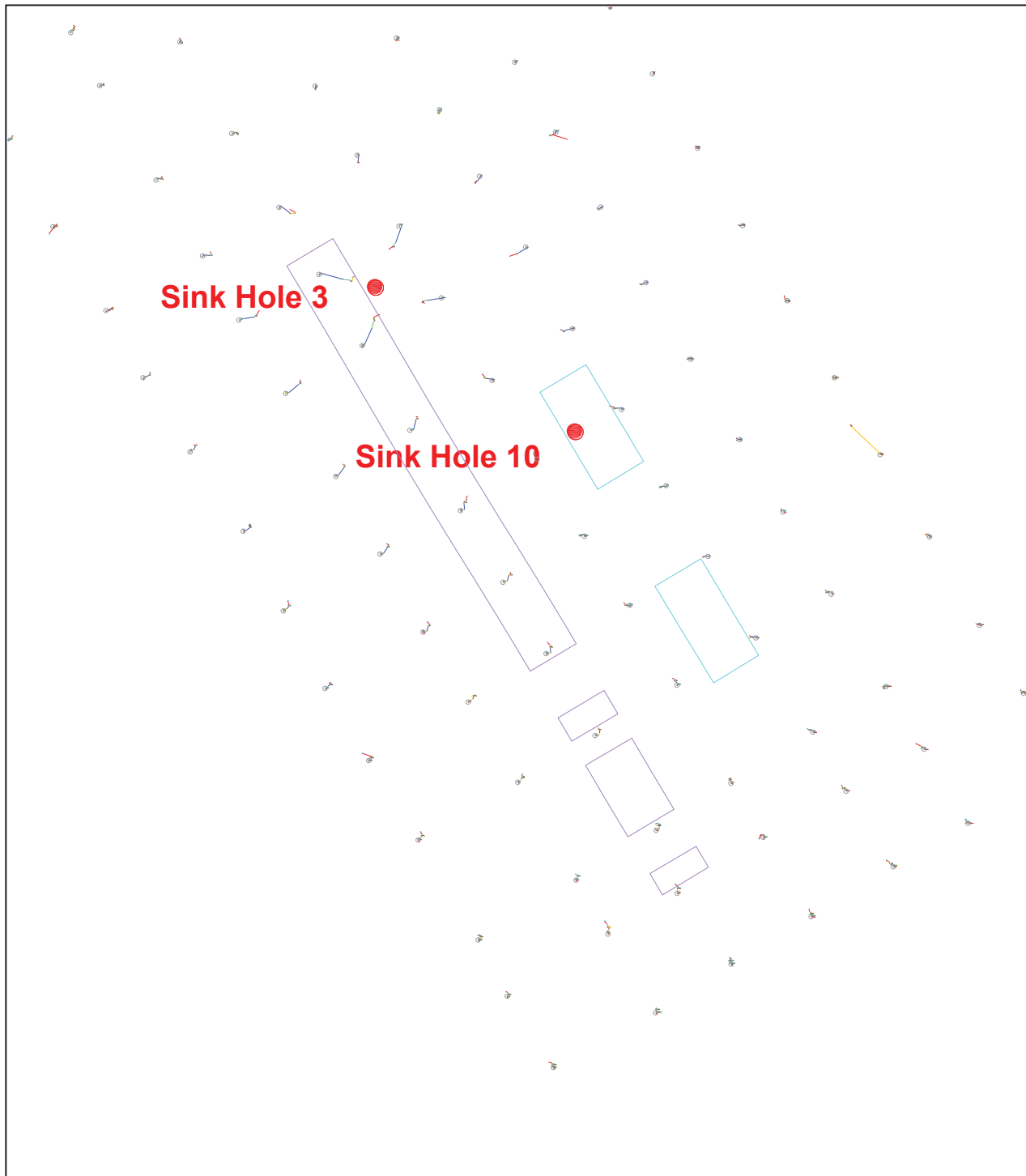
Fig. 6.5 Loci of horizontal movement at survey prisms – far end (south)
