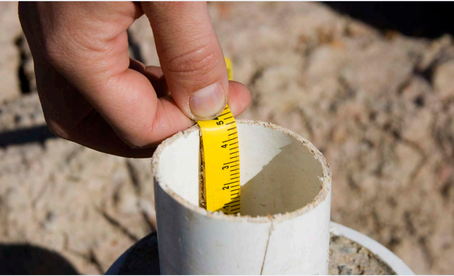
Close up of a piezometer used for measuring groundwater level
