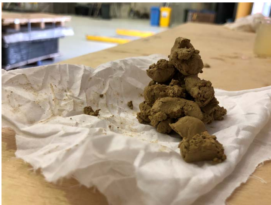
Figure 6: Cake at approximately 70% wt suspended solids
