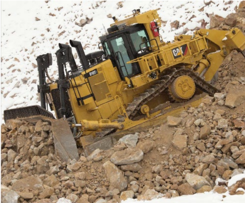
Figure 10: D10 Caterpillar Dozer
