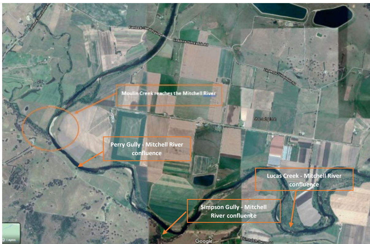
Figure 17: Dam failure has only been modelled for reaching the Mitchell via Moulin Creek. There are other possible paths too that must be considered.
