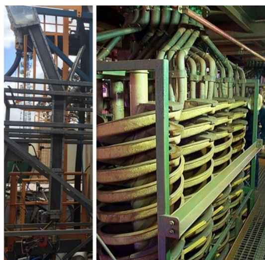
Figure 1 Separation test work has been carried out using a laboratory scale FLSmidth RC100 reflux classifier (left) and full scale Mineral Technologies MG12 spiral (right)
